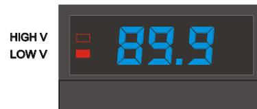
The HIGH V indicator will illuminate when the output voltage is 121.0 VAC or higher. The indicator will remain illuminated until the voltage drops to 120.0 VAC or lower.
