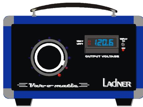
The *Var-o-matic* is a non-isolated 1KVA continuously variable autotransformer capable of adjusting the output AC voltage between 0% and 120% of the input line voltage that it is connected to. Integrated digital voltage meter, with preset high and low limits, give the user the output voltage at a glance. All interconnects are mounted on the rear panel.
